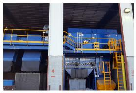
The changes at the Mid America Recycling facility in Lincoln, Neb. have increased throughput from about 1.5 tons per hour up to 10 to 12 tons per hour.
